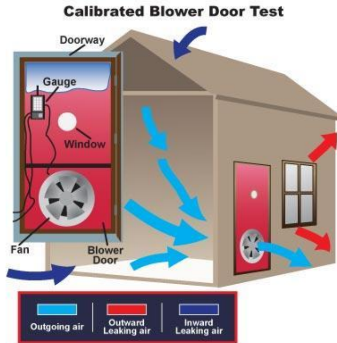
Figure 3 – Forced air is blown out of the house in the leaks and cracks of the exterior.
